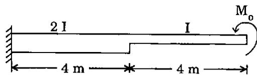
A cantilever beam as shown in figure is subjected to end moment  $M_o$ . What is the deflection at the free end?
