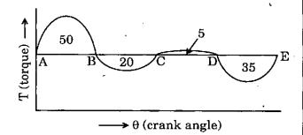
The crank-effort diagram of an engine running a machine is showing the areas above and below the mean line (in joules). What is the maximum fluctuation of energy in the above diagram?
