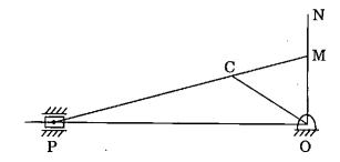
OCP is a slider-crank mechanism. OC = 10 cm is the crank. CP is the connecting rod = 22 cm; OP = 30 cm. ON is perpendicular to OP. PC extended meets ON at M. OM = 7.5 cm, CM = 8.0 cm. Crank runs at 10 rad/s. Find the velocity of the piston in cm/s.
