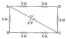
What is the potential difference between the points A and B in the circuit given above?
