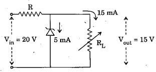
A zener voltage-regulator circuit is shown above. What is the value of the limiting resistor R?
