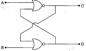
In the above circuit, if the inputs A = B = 0, then what are the possible logic states of C and D respectively?
