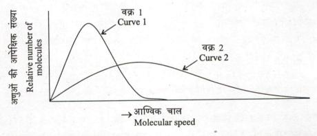
The graph above shows the distribution of molecular speeds for Argon and Helium at the same temperature.
