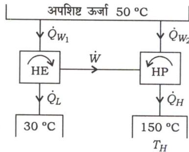
A combination of a heat engine driving a heat pump (see the figure) takes waste energy at  $50^\circ\text{C}$  as a source,  $\dot{Q}_{W_1}$ , to the heat engine rejecting heat at  $30^\circ\text{C}$ . The remainder,  $\dot{Q}_{W_2}$ , goes into the heat pump that delivers  $\dot{Q}_H$  at  $150^\circ\text{C}$ . If the total waste energy is 5 MW, find the rate of energy delivered at the higher temperature. Assume heat engine and heat pump as reversible :
