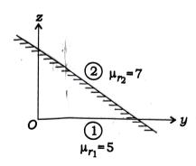
In the figure given below, region 1 is the side of the plane y+z=1 containing the origin and in this region,  $\mu_{r_1}=5$ . In region 2,  $\mu_{r_2}=7$ . It is given that  $\vec{B}_1=3.0\vec{a}_x+1.0\vec{a}_y$  (T). Determine  $\vec{B}_2$  and  $\vec{H}_2$ . Given,  $\mu_0=4\pi\times10^{-7}$ H/m:
