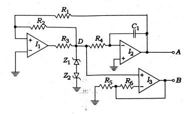
Suggest to replace suitable resistances so that the output voltages at A and B are having swing of  $\pm 6$  V and the output frequency is fixed to 500 Hz.
