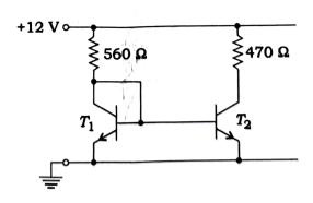
In the circuit diagram given here,  $T_1$  and  $T_2$  are transistors with matched characteristics. The transistor parameters in active region are  $\beta = 200$  and  $V_{BE} = 688$  mV. Find  $V_{CE}$  of transistor  $T_2$ :
