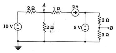
Find the voltage on points A and B of the given circuit:
