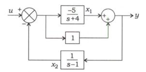
Write the state and output equations for the system shown in the figure. Choose state variables  $x_1$  and  $x_2$  as shown in the figure. Check the controllability and observability of the system:
