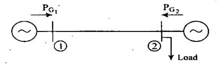
If 100 MW power is transferred from plant 1 to load, a loss of 12 MW is incurred. System incremental cost is  $\lambda = \text{Rs. } 30/\text{MWh}$ . The incremental costs of the two plants are given by:
