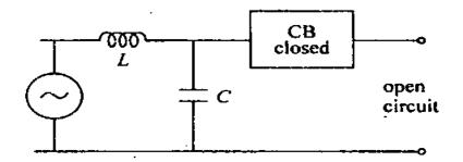
A fault occurs at the far end of the system and the breaker contacts separate. Derive an expression for the voltage across the breaker contacts. Find the frequency of oscillation of the recovery voltage. What is the highest value of the Restriking Voltage and when does it occur.
