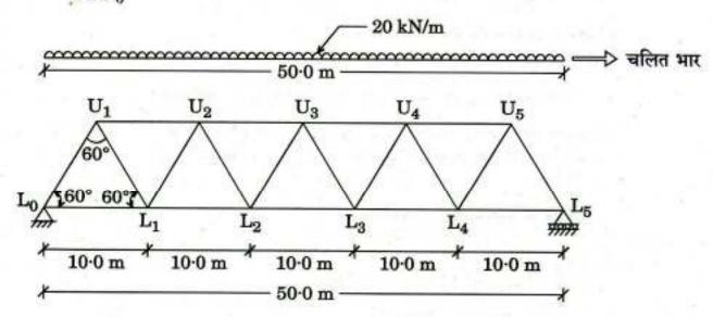
Calculate maximum force in the diagonal member  $U_2L_2$  of the truss shown in the figure below, for a moving load of 20 kN/m (intensity) and 50.0 m in length. It is proposed that this moving load will be transmitted through the bottom chord. (Neglect the self-weight of truss)
