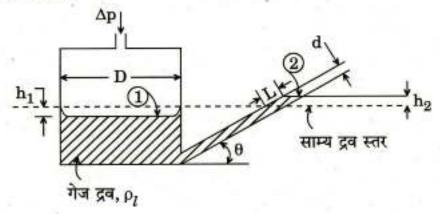
An inclined tube reservoir manometer is constructed as shown. Derive a general expression for the liquid deflection, L, in the inclined tube, due to the applied pressure difference,  $\Delta p$ .
