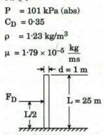
A cylindrical chimney 1 m in diameter and 25 m tall is exposed to a uniform 50 km/h wind at standard atmospheric conditions. End effects and gusts may be neglected. Estimate the bending moment at the base of the chimney.
