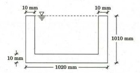
Channel section shown in the figure is carrying water to full depth.
