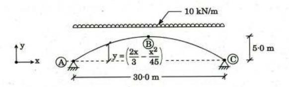
A three-hinge parabolic arch,  $y = \frac{2x}{3} - \frac{x^2}{45}$  has a span of 30·0 m and maximum rise of 5·0 m at centre. Arch is having uniform cross-section throughout. It is subjected to uniformly distributed load of 10 kN/m (dead load + live load).
