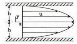
The velocity distribution for the flow of a Newtonian fluid between two fixed wide, parallel plates is given by the following equation:
