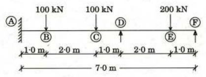
Calculate the value of Plastic Moment 'Mo,' for the beam shown below. 20
