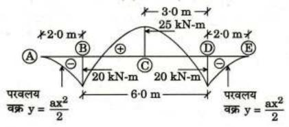
Bending moment diagram for a beam carrying uniformly distributed load has been shown below. Bending moment diagram curve is parabolic and follows the equation  $y = \frac{ax^2}{2}$  in AB and DE portion.
