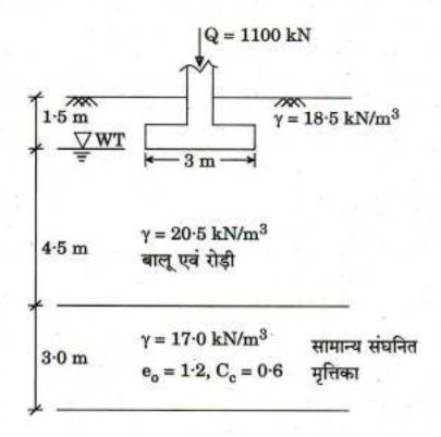
A square footing of size  $3 \text{ m} \times 3 \text{ m}$  is placed on a sand and gravel layer at a depth of 1.5 m from the ground surface. Below the sand and gravel layer, a layer of normally consolidated soil of thickness 3 m is present. Details of soil properties and the footing loading are shown in the figure. Determine the total expected consolidation settlement for the clay layer because of the footing loading.
