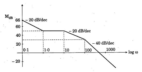
An approximate Bode plot of magnitude for a system was obtained and is shown below. Identify the system in terms of minimum phase transfer function.
