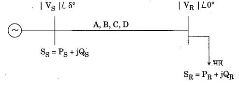
For a 2-bus system shown below, derive expressions for Real Power and Reactive Power at receiving end and sending end.
