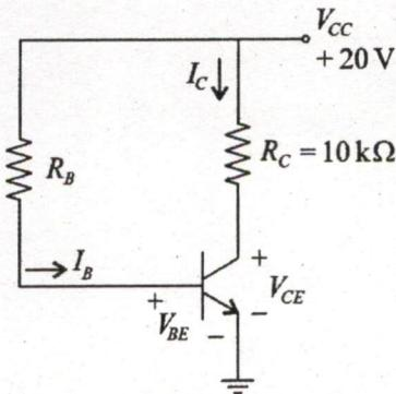
Sketch the dc load line for the circuit shown.
